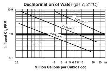
**Empty Bed Contact** BedVolume (ft<sup>3</sup>) x 7.481 gal/ft<sup>3</sup> Time in Minutes Flowrate (gpm)
